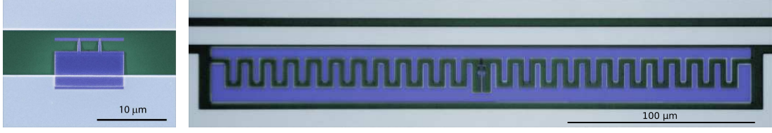
Figure 2.6: Comparison of the geometry of a conventional split CPB (left) and a transmon (right).
