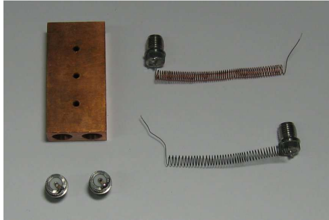
Figure 6.10: Different parts of the powder filter: The copper mount, copper and constantan wires wound into a coil with and soldered to a press-fit SMA connector with an additional capacitance soldered between the center pin and the ground.
